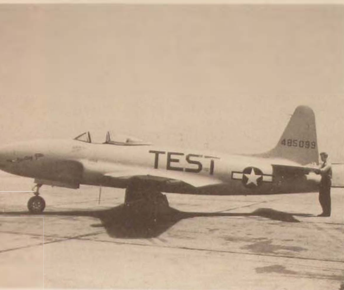
America's first combat-worthy swing-role jet fighter, the P-80, was a typical first-generation jet warplane, blending the established aerodynamics of the subsonic propeller-driven airplane with the revolutionary jet engine.
