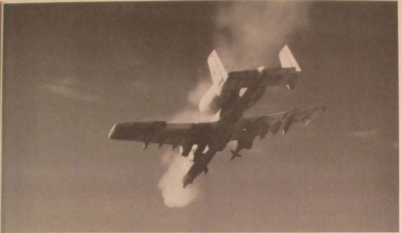
The internally mounted GAU-8 30-mm Gatling gun is the most notable feature of the A-10, providing it with immense firepower.
